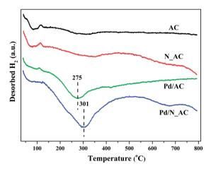
Fig. 5 H<sub>2</sub>-TPD profiles of AC, N\_AC, Pd/AC and Pd/N\_AC.
