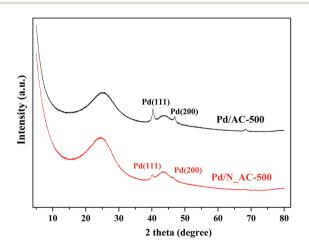
Fig. 6 XRD patterns of Pd catalysts after calcined at 500 °C.
