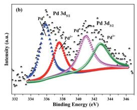
Pd 3d XPS spectra of (a) Pd/AC and (b) Pd/N\_AC
