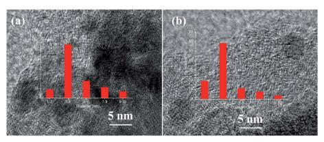
Fig. 4 HRTEM images and size distribution of (a) Pd/AC and (b) Pd/N\_AC.
