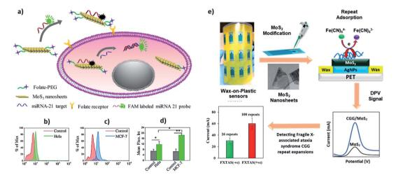
Fig. 6 (a-d) Interface of ssDNA-MoS<sub>2</sub>-PEG-FA probe-based FRET platform for intracellular miRNA-21 detection in cancer cells, i.e. HeLa and MCF-7 cells. Reprinted with permission from ref. 85 with copyright (2018) American Chemical Society. (e) Label-free electrochemical detection of fragile X-associated repeats (CGG repeats) on MoS<sub>2</sub> nanosheets modified wax-on-plastic platforms. Reprinted with permission from ref. 86 with copyright (2020) American Chemical Society.
