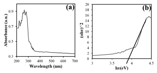
Fig. 5 Graphs of (a) DRS and (b)  $(\alpha hv)^2$  versus hv for the band gap estimate obtained from sample no. 3.
