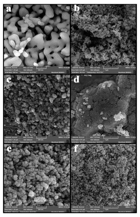
Fig. 2 SEM images of nanoparticles synthesized by the ultrasonic method with (a and b)  $NH_3$  as a pH adjustment agent, (c and d) en as a pH adjustment agent and 5 min under ultrasonication, and (e and f) en as a pH adjustment agent and 10 min under ultrasonication.
