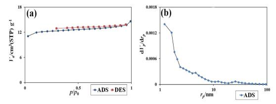
Fig. 11 (a) The isotherm obtained from the study of  $N_2$  adsorption/desorption on  $Tl_4Hgl_6/Hgl_2$  nanocomposite, (b) the graph obtained from BJH calculations of sample no. 8.
