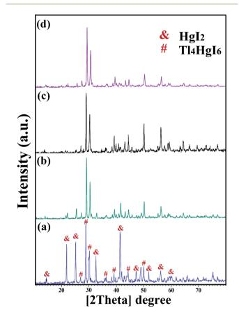
Fig. 1 XRD patterns obtained from  $Tl_4Hgl_6/Hgl_2$  nanocomposite in different ratios of Tl to  $Hgl_2$  precursors; (a) 1:1, (b) 2:1, (c) 3:1, and (d) 1:2.
