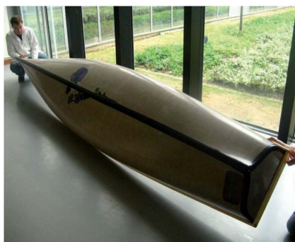
Fig. 2 Flax/PLA canoe manufactured during the NAVECOMAT project.
