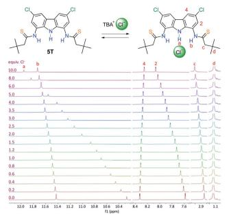
Fig. 2  $\,^{1}$ H NMR titration of **5T** (5 mM) with TBACl in DMSO- $d_{6}$  + 0.5% H<sub>2</sub>O. T = 293 K.
