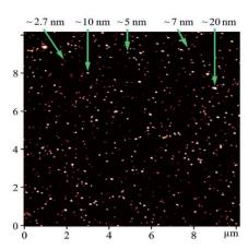
Fig. 2 AFM image of  ${\rm WS}_2$  particles deposited on mica substrate. Numbers with arrows show the height of objects.
