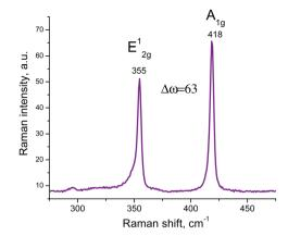
Fig. 4 Raman spectrum of the 2D WS<sub>2</sub> nanoparticles.
