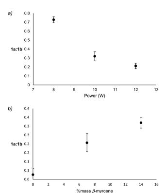
Fig. 5 The relationship between applied power to 1a:1b (a) and % mass  $\beta$ -myrcene to 1a:1b (b). 1a:1b is calculated as the quotient of the selected ion chromatogram integrations of the molecular ions for 1a products, 3MCA (m/z=84 amu) and 2M2B (m/z=70 amu), with 1b products, isoprene (m/z=67 amu) and 3M1B (m/z=70 amu).
