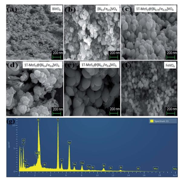
Fig. 3 SEM analysis for (a) pure BiVO<sub>4</sub>, (b)  $(Bi_{0.5}Fe_{0.5})VO_4$ , (c) 1T-MoS<sub>2</sub>@ $(Bi_{0.75}Fe_{0.25})VO_4$ , (d) 1T-MoS<sub>2</sub>@ $(Bi_{0.20}Fe_{0.80})VO_4$ , (e) 1T-MoS<sub>2</sub>@ $(Bi_{0.40}Fe_{0.60})VO_4$ , and (f) pure FeVO<sub>4</sub>. (g) EDX analysis of 1T-MoS<sub>2</sub>@ $(Bi_{0.40}Fe_{0.60})VO_4$  heterostructures.
