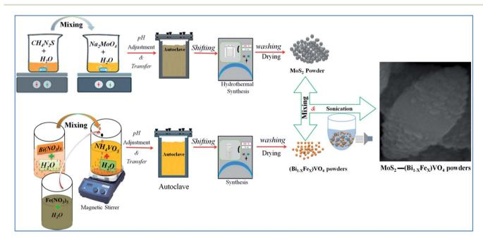
Fig. 1 Schematic representation of experimental setup for preparation of 1T-MoS<sub>2</sub> decorated on the surface of (Bi<sub>1-x</sub>Fe<sub>x</sub>)VO<sub>4</sub>.
