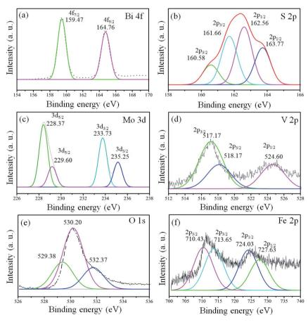
Fig. 4 High-resolution peak-fitting XPS spectra of (a) Bi 4f, (b) S 2p, (c) Mo 3d, (d) V 2p, (e) O 1s and (f) Fe 2p of 1T-MoS<sub>2</sub>@(Bi<sub>0.40</sub>Fe<sub>0.60</sub>)VO<sub>4</sub> heterostructures.
