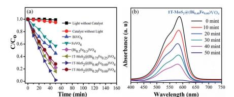
Fig. 5 (a) Degradation of CV dye solution under different conditions; (b) UV-visible absorption spectra of CV dye solution during photocatalytic degradation over  $1T-MoS_2@(Bi_{0.40}Fe_{0.60})VO_4$  heterojunction photocatalysts at different time intervals.
