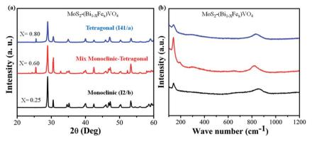
Fig. 2 (a) XRD patterns and (b) Raman spectra for the 1T-MoS<sub>2</sub>@(Bi<sub>1-x</sub>Fe<sub>x</sub>)VO<sub>4</sub> nanoparticles synthesized at 180 °C
