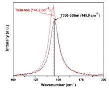
Fig. 3 Raman spectra of samples T530-550 and T530-550im illustrating the shift of the main  $E_{\alpha}$  peak from the presence of sulphur ions.
