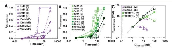
Fig. 3 NMR yield of phenanthrene evolution for (A) iodine- and (B) TEMPO-oxidized systems; (C) concentration dependence of phenanthrene formation at 2 h (light lines and symbols) and 16 h (dark lines and symbols). Dotted line represents complete conversion.
