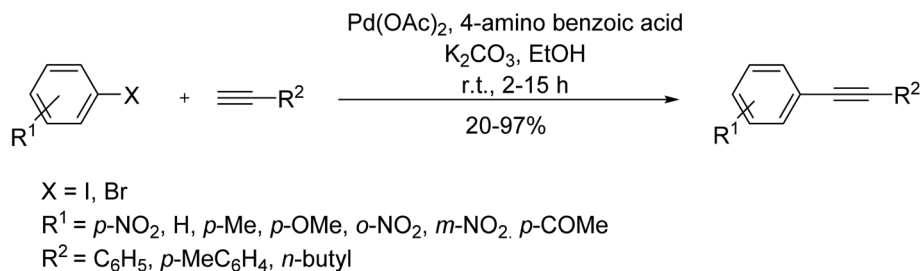
Scheme 25 Copper-free Sonogashira coupling reactions in the presence of the \text{Pd(OAc)}_2 .
