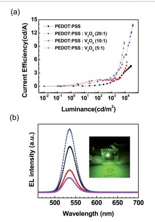
**Fig. 5** (Color online) (a) Current efficiency–luminance characteristics and (b) EL spectra of QLED devices at each maximum luminance. The inset shows an image of the device operating.
