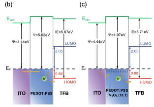
Fig. 1 (Color online) (a) UPS spectra of ITO, ITO/HILs and ITO/HILs/TFB measured near the SEC (left) and  $E_{\rm F}$  region (right). The inset represents the area under the UPS spectra near the  $E_{\rm F}$  of PEDOT:PSS (gray) and PEDOT:PSS:  $V_2O_5$  (10 : 1) (blue). Interfacial energy level diagram of (b) ITO/PEDOT:PSS/TFB and (c) ITO/PEDOT:PSS:  $V_2O_5$  (10 : 1)/TFB.
