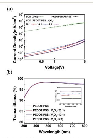
Fig. 3 (Color online) (a) Current density–voltage (J-V) characteristics of the HODs (ITO/HIL/TFB/Al) and EOD (ITO/ZnO/Al). (b) Transmittance of different HIL films on glass substrate. The inset shows the transmittance in the range of 530 to 540 nm.
