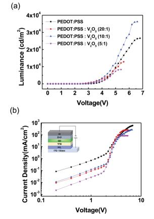
Fig. 4 (Color online) (a) Luminance–voltage (L-V) curves of the QLED devices. (b) J-V characteristics of the QLED devices with different HIL. The inset shows the schematic diagram of QLED device.
