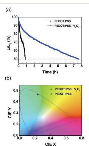
Fig. 6 (Color online) (a) Operational lifetime and (b) CIE 1931 coordinate of QLED devices with PEDOT:PSS and PEDOT:PSS:  $V_2O_5$  (10:1).
