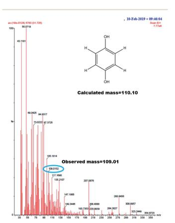
Fig. 10 GC-MS of PhOCH<sub>3</sub>-Redox showing m/z = 109.01, Ph-(OH)<sub>2</sub> (hydroquinone; M-H peak) (calculated, 110.10).
