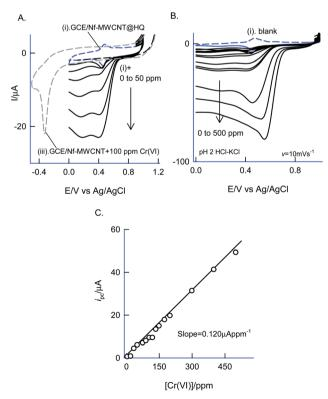
Fig. 12 (A and B) CV responses of GCE/Nf–MWCNT@HQ (Ph-OCH<sub>3</sub>-Redox) without (curve (i)) and with various concentrations of  ${\rm Cr_2O_7}^{2-}$  (curve (ii)) at v=10 mV s<sup>-1</sup> in pH 2 KCl–HCl buffer. Curve (iii) is a control CV response of GCE/Nf–MWCNT with 100 ppm of  ${\rm Cr_2O_7}^{2-}$  in pH 2 KCl–HCl solution. (C) Calibration plot of (C)  $i_{\rm pc}$  vs.  ${\rm Cr_2O_7}^{2-}$  concentration.
