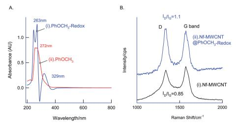
Fig. 8 Physicochemical characterization of the Nf–MWCNT@PhOCH<sub>3</sub>-Redox with control samples using (A) Raman spectra and (B) UV-Vis spectroscopic techniques. For UV-Vis analysis of PhOCH<sub>3</sub>-Redox, an ethanol extract GCE/Nf–MWCNT@PhOCH<sub>3</sub>-Redox followed by column filtered sample was used. Screen-printed electrode modified was used for Raman spectroscopic analysis.
