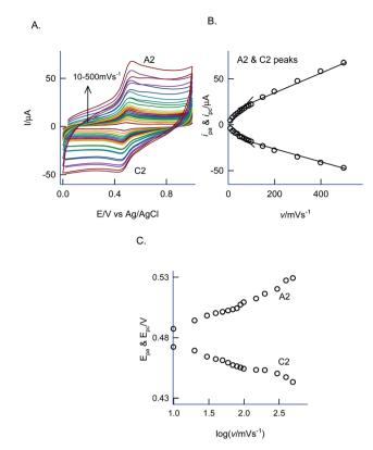
Fig. 2 (A) CV response of effect of scan rate (10–500 mV s $^{-1}$ ) on GCE/Nf–MWCNT@PhOCH $_3$ -Redox in pH2 KCl–HCl buffer. Plots of (B) anodic peak current ( $i_{\rm pa}$ ) and cathodic peak current ( $i_{\rm pc}$ ) vs. scan rate and  $E_{\rm pa}$  and  $E_{\rm pc}$  vs. log of scan rate (C) for A2/C2 peak.
