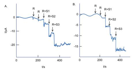
Fig. 14 Amperometric i-t based real sample analysis of Cr(vi) species in two industrial effluents samples using GCE/Nf-MWCNT@HQ modified electrode in pH 2 KCl-HCl solution. A four-time diluted test sample with pH 2 KCl-HCl was subjected for the analysis.  $E_{app} = 0.4 \text{ V vs. Ag/AgCl. R} = \text{real sample, R} + \text{S1-S3} = \text{real} + \text{three different standard Cr(vi) concentration numbers, 1-3.}$
