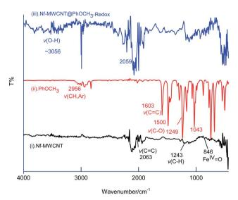
Fig. 9 Comparative FTIR characterization responses of Nf–MWCNT (curve (ii)), PhOCH $_3$  (curve (iii)), Nf–MWCNT@PhOCH $_3$ -Redox (curve (iii)).
