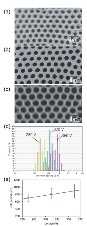
Fig. 5 SEM images of long-range ordered anodic porous alumina formed at different voltages: (a) 280, (b) 320, and (c) 360 V. (d) Interhole spacing distributions of the obtained samples. (e) Relationship between the inter-hole spacings and applied voltages.
