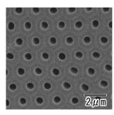
Fig. 6 SEM image of ordered anodic porous alumina obtained at 600 V. The anodization was carried out in an electrolyte with a mixture of water and ethylene glycol (1:1 volume ratio) containing 25 mM citric acid and 0.15 mM phosphoric acid at 16 °C for 160 h. The thickness of the sample was 50 µm.
