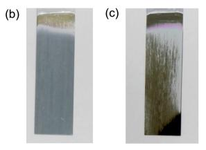
Fig. 1 (a) Current–time curves obtained during the anodization of an Al sheet in 0.2 M citric acid electrolytes with and without 3 mM phosphoric acid at 10  $^{\circ}$ C. Photographs of samples obtained in 0.2 M citric acid electrolytes with (b) and without (c) 3 mM phosphoric acid.
