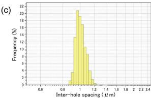
Fig. 2 SEM image of highly ordered anodic porous alumina obtained at 400 V; (a) surface and (b) cross-sectional views. The first anodization was carried out in 0.2 M citric acid and 3 mM phosphoric acid at  $10\,^{\circ}$ C for 48 h. (c) Inter-hole spacing distribution of the obtained sample.
