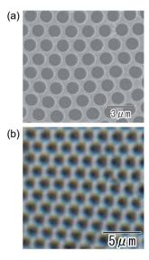
Fig. 7 SEM (a) and optical microscope (b) images of highly ordered anodic porous alumina obtained at 700 V. The anodization was carried in an electrolyte with a mixture of water and tetraethylene glycol (1:1 volume ratio) containing 25 mM citric acid and 0.25 mM phosphoric acid at 16 °C for 550 h. The thickness of the sample was 280  $\mu m$ .
