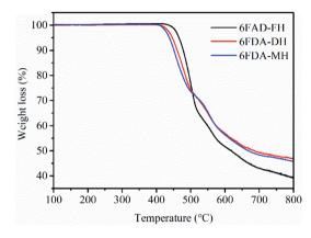
Fig. 4 TGA curves of the three Pls under N<sub>2</sub>.
