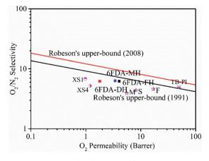
Fig. 8 Robeson's upper bounds relevant to the three PIs (6FDA-FH, 6FDA-DH, and 6FDA-MH) for  $CO_2/CH_4$  and  $O_2/N_2$ . The data points are those of XS1,<sup>48</sup> XS4,<sup>48</sup> M (6FDA-MSBC),<sup>22</sup> F (6FDA-FSBC),<sup>22</sup> S (6FDA-SBC),<sup>22</sup> and TB-PI.<sup>46</sup>
