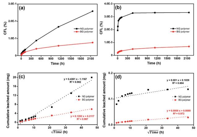
Leaching behavior of (a and c) Cs and (b and d) Co from NG and BG polymer waste forms. The data were collected up to 90 d (2160 h).
