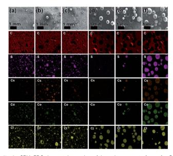
Fig. 2 SEM-EDS elemental mapping of the polymer waste forms for C, S, Cs, Co, and Cl elements: (a–c) represent the elemental mapping for BG polymer waste from top, middle, and bottom sections, respectively; (d–f) display the elemental mapping for NG polymer waste from top, middle, and bottom sections, respectively.
