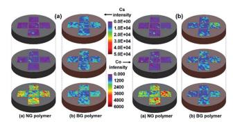
Fig. 1 2D mapping of the simulated NG and BG polymer waste forms by LIBS analysis. Polymer waste forms were equally divided into three sections: top, middle, and bottom for (a) Cs and (b) Co distribution.
