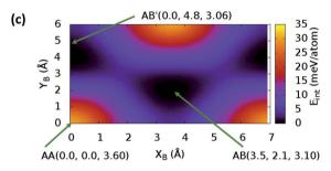
Fig. 2 Stacking energy profile for (a) bulk  $C_{12}H_6$ -h2D, (b) bulk  $B_6N_6H_6$ -h2D, and (c) bulk  $C_6N_6$ -h2D. ( $X_B$ ,  $Y_B$ ) is the shift in the top layer relative to the bottom layer. ( $X_B = 0$ ,  $Y_B = 0$ ) corresponds to the AA stacking. AB' denotes the most stable stacking in  $C_6N_6$ -h2D, which corresponds to neither AA nor AB.  $E_{\rm int}$  values presented are relative to the most stable stacking configuration.
