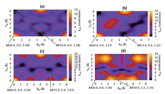
Fig. 3 Stacking energy profile in (a) bulk  $C_{10}N_2H_4$ -o2D, (b) bulk  $C_8N_4H_2$ -o2D, (c) bulk  $C_{10}P_2H_4$ -o2D, and (d) bulk  $C_{10}As_2H_4$ -o2D. ( $X_B$ ,  $Y_B$ ) represents the shift in the top layer relative to the bottom layer. ( $X_B = 0$ ,  $Y_B = 0$ ) corresponds to the AA stacking.  $E_{int}$  values presented are relative to the most stable stacking configuration.
