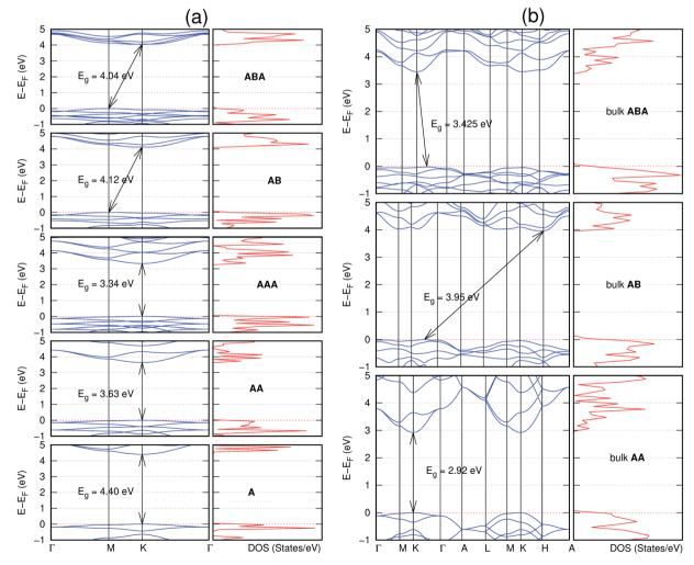
Fig. 11 Effect of stacking on the electronic structure of  $B_6N_6H_6$ -h2D for (a) isolated one, two, and three layers with the specified stackings and (b) the bulk system with the specified stackings. The fundamental band gap is marked with an arrow that indicates their direct or indirect nature. The Fermi level is set at the top of the valence band.
