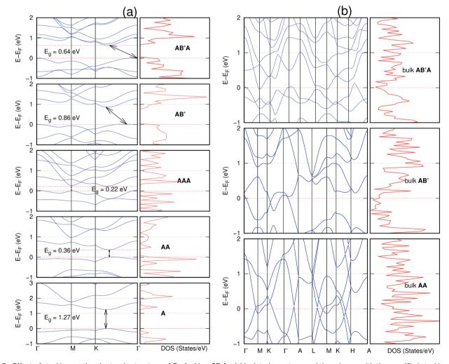
Fig. 7 Effect of stacking on the electronic structure of  $C_{10}$ As<sub>2</sub>H<sub>4</sub>-o2D for (a) isolated one, two, and three layers with the specified stackings and (b) the bulk system with the specified stackings. The fundamental band gap is marked with an arrow that indicates their direct or indirect nature. The stacking AB' indicates that the most stable stacking corresponds to neither AA nor AB. In semiconducting systems, the Fermi level is set at the top of the valence band.
