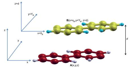
Fig. 1 Bilayer stacking scheme. Cartesian coordinates of the atoms in the bottom layer are fixed at A(x,y) while those for the top layer are  $B(x+X_B, y+Y_B)$ .  $X_B$  and  $Y_B$  vary from 0 to a full lattice constant a and b sin  $\gamma$ , respectively so that  $B(x+a,y+b\sin\gamma)$  corresponds to a full lattice mismatch of B relative to A.
