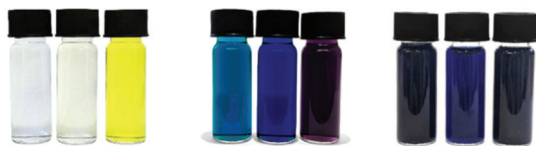
Fig. 6 From left to right: photographs of the solutions of parent compounds 5 , 6 , and 7 in dichloromethane ( c = 5.5 \times 10^{-4} M, left), hexachloroantimonate salts of 5^+ , 6^+ , and 7^+ in dichloromethane ( c = 5.5 \times 10^{-4} M, center) and of 5^{2+} , 6^{2+} , and 7^{2+} in nitromethane ( c = 5.5 \times 10^{-4} M, right).
