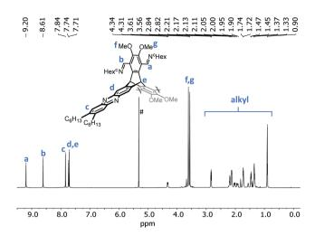
Fig. 3 <sup>1</sup>H NMR spectrum (700 MHz, CD<sub>2</sub>Cl<sub>2</sub>) of cage (R,R)-9. # residual CH2Cl2.
