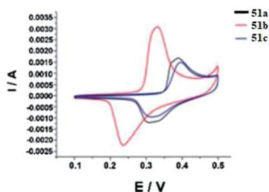
Fig. 3 Cyclic voltammetry (CV) curves for compounds **51a–c**, the obtained samples in 2 M KOH electrolyte versus SCE at a scan rate of  $20 \text{ mV s}^{-1}$ , the voltage window ranged from 0.0–0.5 V. Adapted from ref. 43 with permission from The Royal Society of Chemistry.
