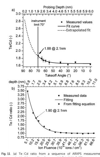
Fig. 11 (a) Te:Cd ratio from a sequence of ARXPS measurements compared with (b) a profile of sequential 5 keV Ne<sup>+</sup> ISS measurements as a comparison probe of the two methods efficacy in the analysis of ultrathin films.<sup>216</sup>
