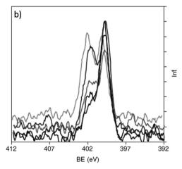
Fig. 8 (a) N 1s spectrum of PMG recorded on a MnOOH surface at room temperature versus fast frozen, evidencing an addition nitrogen species following preparation via cryo-transfer. (b) N 1s spectrum of PMG on MnOOH at pH 3.9, 4.9, 6.0, 7.9 and 8.6 (top to bottom spectral features at around 402 eV). Here we can see the pH dependence on the amount of protonated PMG species on the surface of MnOOH. Copyright © 2004 John Wiley & Sons, Ltd.<sup>135</sup>
