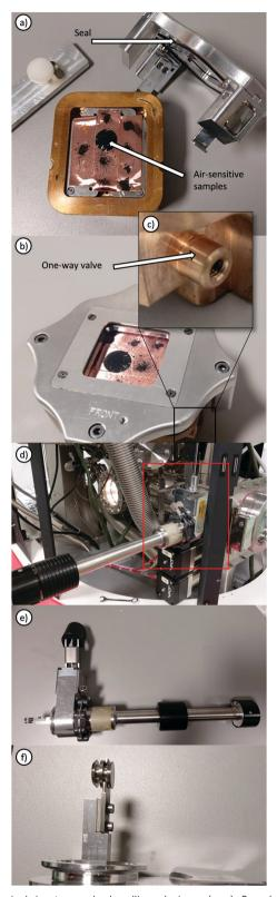
Fig. 4 Typical inert sample handling devices. (a-c) Sample transfer under vacuum from Thermo Scientific<sup>TM</sup>. (a) Disassembled transfer unit, (b) assembled transfer unit and (c) check valve to hold internal vacuum – (d-f) sample transfer under vacuum or inert gas from Kratos Analytical. (d) Transfer arm attached to UHV chamber, (e) transfer arm removed from UHV chamber and (f) sample stub held on manipulator probe.
