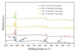
Fig. 9 Survey spectra of copper activated sphalerite after; no etching, 2 minutes, 4 minutes, and 6 minutes of etching corresponding to a depth of 3, 6, 10 nm respectively Reprinted from Ejtemaei et al., Characterisation of sphalerite and pyrite surfaces activated by copper sulfate, Miner. Eng., 2017, 100, 223-232, Copyright (2007), with permission from Elsevier.148
