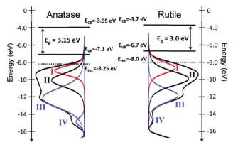
Fig. 14 He(I) UPS profiles, fit with an established empirical model and an overlayed electronic structure of the two TiO2 polymorphs anatase and rutile relative to the vacuum level.  $E_{\rm thr.}$  corresponds to the deepest state that can be excited in a photocatalytic test ( $E_{\rm photons} \leq 4.3$  eV).<sup>262</sup>
