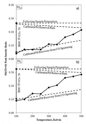
Fig. 12 Pd/(Ti + O) ISS intensity ratios for  $Pd_{20}/TiO_2$  (a) and  $Pd_2/TiO_2$ (b) as-deposited, after exposure to CO at 180 K, and during temperature ramping. Calibrated rates for recovery of Pd from ISS sputtering.<sup>171</sup> Calibration lines account for unintended sputtering effects from the ISS experimental conditions selected for this analysis. Deviations from this calibration indicate a changing surface structure (desorption of CO)
