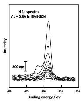
Fig. 6 XPS depth profiling spectra of the N 1s level from Mn oxide electrodes in EMI-SCN, [C2C<sub>1</sub>Im][SCN] polarised at -0.3 V, reported by Chang et al. Reprinted (adapted) with permission from ref. 122. Copyright {2009} American Chemical Society.
