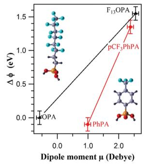
Fig. 15 Correlation between the experimental change in work function  $(\Delta \Phi)$  and the molecular dipole moment  $\mu$  of the PA molecules for 3,3,4,4,5,5,6,6,7,7,8,8,8-tridecafluorooctyl phosphonic acid-((F<sub>13</sub>)OPA, left molecule in figure) and p-(trifluoromethyl)phenylphosphonic acid-((pCF3)PhPA, right molecule in figure) modified ZnO surfaces, along with corresponding non-fluorinated analogues.<sup>273</sup>
