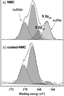
Fig. 5 XPS spectra for the S 2p core peaks after SO<sub>2</sub> adsorption on (a)  $LiCoO_2$  and (a')  $Al_2O_3$  coated  $LiCoO_2$  and XPS spectra for the S 2p core peaks after SO<sub>2</sub> adsorption on (b) NMC and (b') Al<sub>2</sub>O<sub>3</sub> coated NMC. Reprinted (adapted) with permission from ref. 104. Copyright {2015} American Chemical Society.
