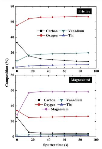
Fig. 3 XPS depth profile composition measurements of pristine and magnesiated V<sub>2</sub>O<sub>5</sub> cathodes indicating the relative contents of carbon, oxygen, vanadium, tin and magnesium as a function of overall ion bombardment time (in itself a function of depth from the surface of the sample down into the bulk).89
