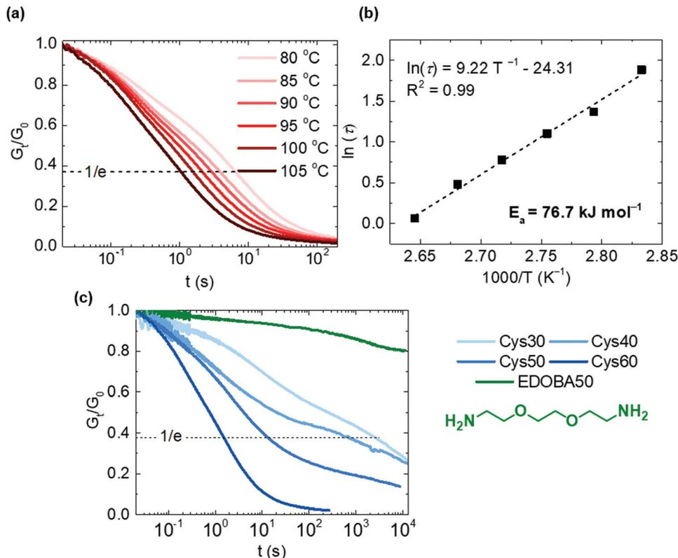
Fig. 4 Dynamic properties of the PA CANs; (a) stress relaxation curves of Cys60 at different temperatures, (b) relaxation times ( $\tau$ ) as a function of the temperature and calculation of the activation energy ( $E_a$ ) for Cys60 and (c) comparison of the stress relaxation of Cys30–60 at 100 °C.
