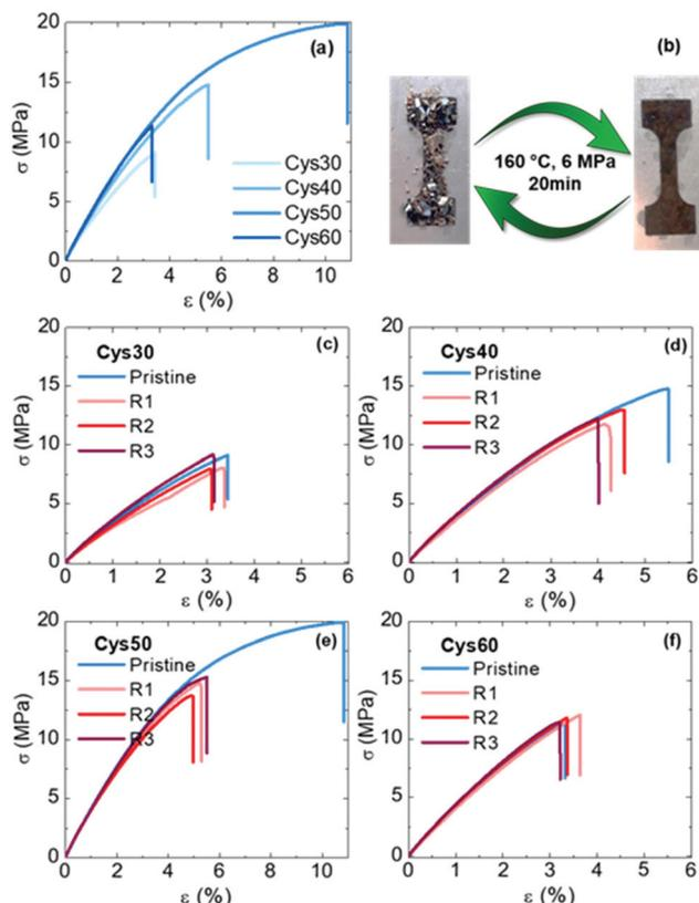
**Fig. 5** Mechanical properties of the PA CANs; (a) stress–strain curves of the pristine networks, (b) appearance of a reprocessed sample after compression molding and (c–f) stress–strain curves of the reprocessed CANs.
