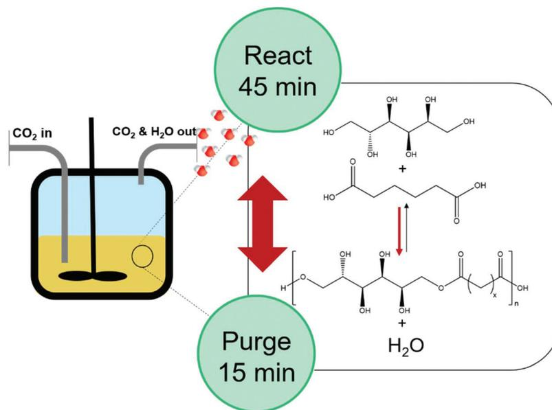
**Fig. 2** Schematic representation of the condensation polymerisation of adipic acid with D-Sorbitol in  $\text{scCO}_2$  in a reactor vessel. The reactor is filled with  $\text{CO}_2$  through an inlet while  $\text{CO}_2$  and  $\text{H}_2\text{O}$  exit through the outlet on the right when the reactor is purged.
