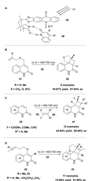
Scheme 10 (A) Hydrogen bond complex formation between chiral thioxanthone 35 and general lactam substrate 36 and (B-D) enantioselective [2 + 2] photocycloadditions in the presence of chiral sensitizer 35.
