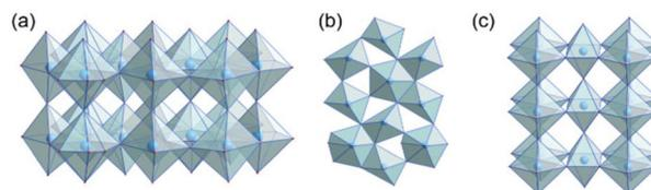
**Fig. 1** (a) Layers in the orthorhombic crystal structure of L-Ta<sub>2</sub>O<sub>5</sub>,<sup>13</sup> (b) connectivity of distorted polyhedra in L-Ta<sub>2</sub>O<sub>5</sub>, and (c) orthorhombic crystal structure of β-Ta<sub>2</sub>O<sub>5</sub>.<sup>14</sup>
