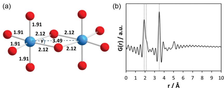
Fig. 2 (a) Model of the dimeric molecular structure of  $\text{Ta}_2(\text{OEt})_{10}$  without the coordinating alcohol molecules as derived from EXAFS data and (b) the resulting calculated PDF. Blue and red spheres represent Ta and O atoms, respectively. The vertical dotted lines are a guide to the eye indicating the maxima of the peaks.
