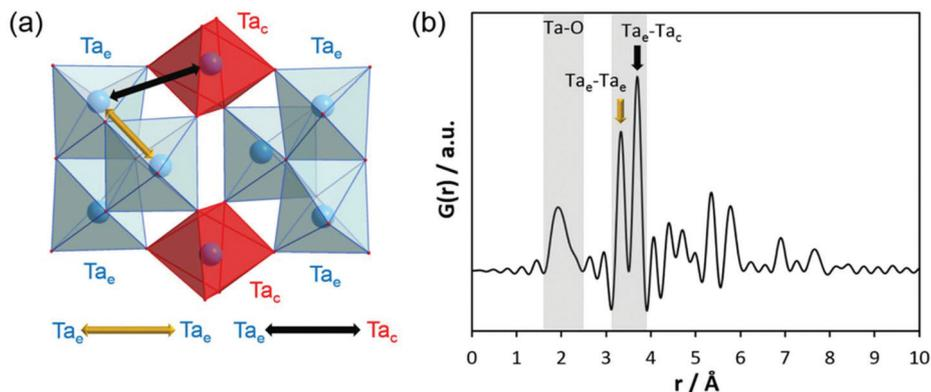
Fig. 4 (a) Model of connected trinuclear units  $[\text{Ta}_8(\mu_3\text{-O})_2(\mu\text{-O})_8(\mu\text{-OEt})_6(\text{OEt})_{14}]$ , based on crystal structure data published for tantalum ethoxide hydrolysed in alcohol by Abrahams *et al.*<sup>50</sup> and (b) simulated PDF of that structure.
