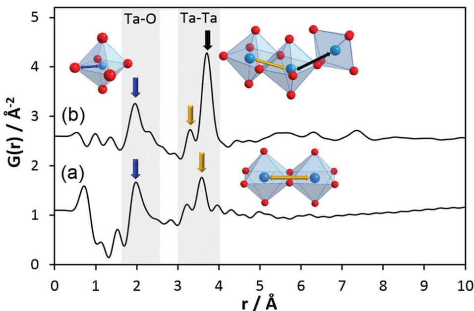
**Fig. 3** Experimental PDFs of (a)  $\text{Ta}_2(\text{OEt})_{10}$  and (b)  $\text{h-Ta}_x\text{O}_y\text{H}_z$ . The main pair correlations are marked by arrows with the blue one representing individual Ta–O distances within an octahedron, the yellow one labels Ta–Ta distances between edge-sharing octahedra, and the black one highlights Ta–Ta distances between corner-sharing octahedra.
