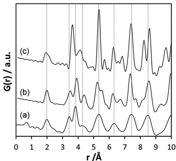
Fig. 10 (a) Experimental PDF obtained at 700 °C during heating of  $d\text{-Ta}_x\text{O}_y$ , calculated PDFs based on the structures of (b)  $L\text{-Ta}_2\text{O}_5$ <sup>13</sup> and (c)  $\beta\text{-Ta}_2\text{O}_5$ .<sup>14</sup>
