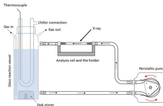
**Fig. 12** Experimental setup used for *in situ* flow cell scattering experiments. The suspension in the glass reaction vessel is pumped through a borosilicate glass cell. The evolving particles are tracked by PDFs obtained from X-ray total scattering data.
