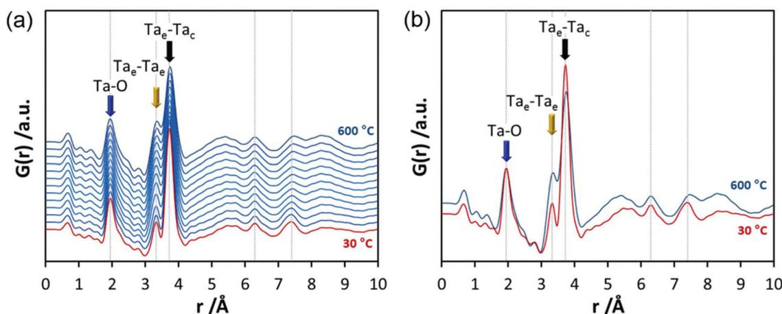
**Fig. 8** (a) Experimental PDFs obtained during heating of d-Ta<sub>x</sub>O<sub>y</sub> from room temperature to 600 °C. (b) Comparison of the experimental PDFs obtained at 30 °C and *in situ* at 600 °C. The atom pairs corresponding to Ta-O distances within the octahedra, between edge-sharing octahedra, and between edge- and corner-sharing octahedra are marked with blue, yellow, and black arrows.
