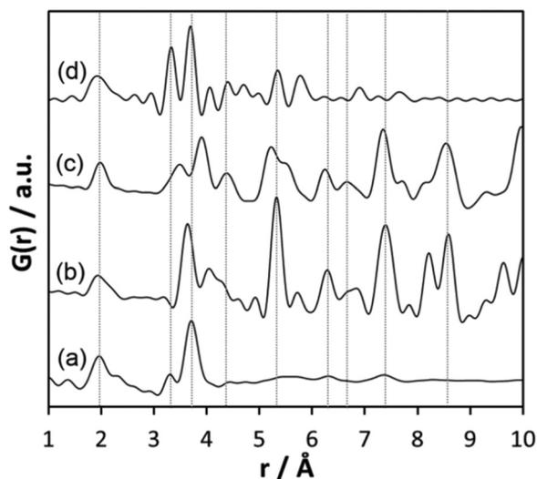
Fig. 5 (a) Experimental PDF obtained from  $h\text{-Ta}_x\text{O}_y\text{H}_z$ , (b) simulated PDF of  $\beta\text{-Ta}_2\text{O}_5$ ,<sup>14</sup> (c) simulated PDF of  $L\text{-Ta}_2\text{O}_5$  structure,<sup>13</sup> (d) simulated PDF based on Abrahams' structure of  $\text{Ta}_8\text{O}_{10}(\text{OEt})_{20}$ .<sup>50</sup>
