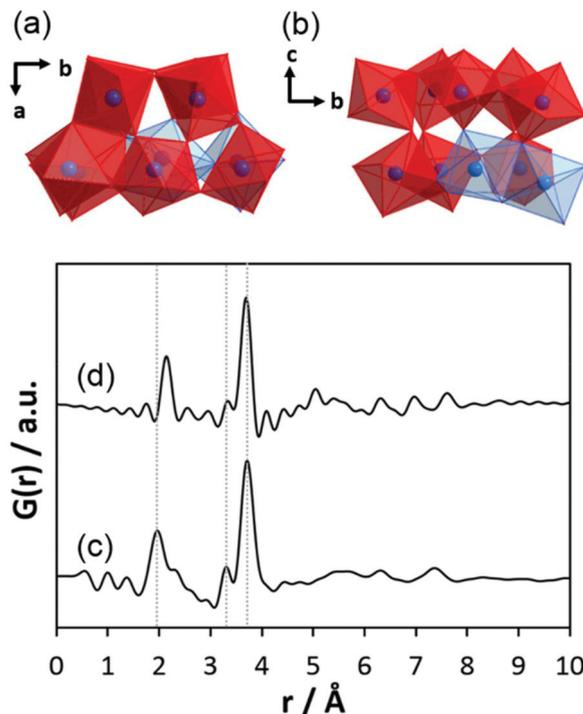
Fig. 11 Cluster model derived from cutting a part of the crystal structure of  $L\text{-Ta}_2\text{O}_5$  followed by a simple geometric optimisation: (a) top view and (b) side view. (c) Experimental PDF of  $h\text{-Ta}_x\text{O}_y\text{H}_z$  is given in comparison to (d) the PDF calculated based on this structure.
