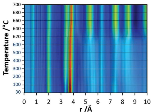
**Fig. 7** False colour heat map of PDFs obtained from *in situ* heating experiments carried out under synthetic air on d-Ta<sub>x</sub>O<sub>y</sub> powder sample. Data for PDF were collected every 50 °C between room temperature and 600 °C and every 10 °C between 600 and 700 °C (red colour indicates high intensities, blue colour low intensity).
