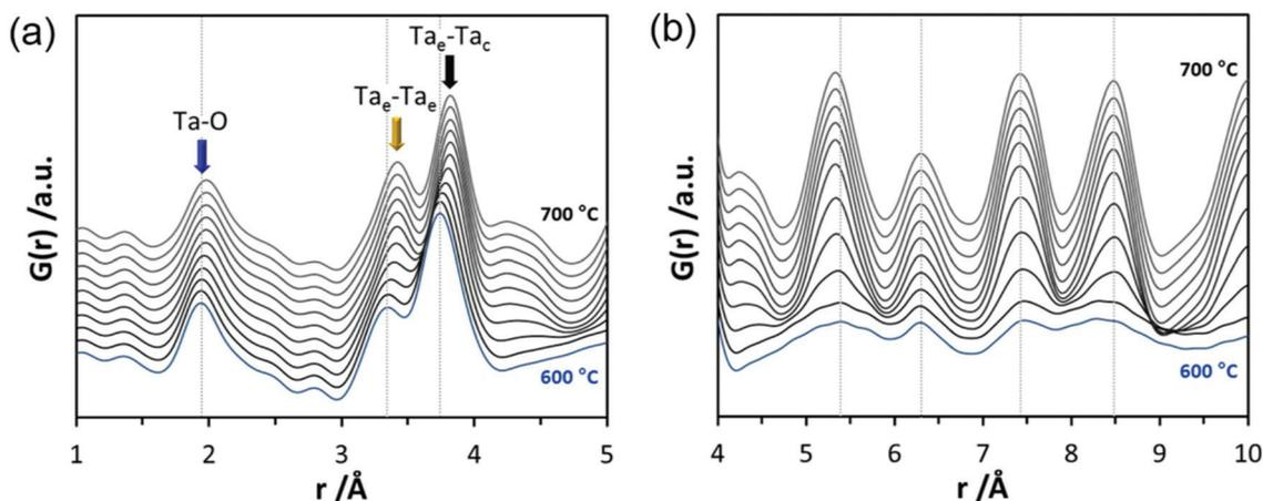
Fig. 9 Experimental PDFs obtained during heating of  $d\text{-Ta}_x\text{O}_y$  between 600 and 700 °C (a) displayed for the  $r$ -range between 1 and 5 Å, (b) in the  $r$ -range between 4 and 10 Å. The atom pairs corresponding to Ta–O distances within the octahedra, between edge-sharing octahedra and between edge- and corner-sharing octahedra are marked with blue, yellow and black arrows.
