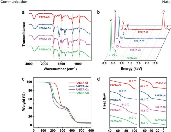
Fig. 2 (a) ATR-FTIR spectra, (b) EDS spectra, (c) TGA curves, and (d) DSC curves (left: dry, right: wet) of PAETA-Cl, PAETA-Ac, PAETA-Ox, and PAETA-Cit hydrogels.
