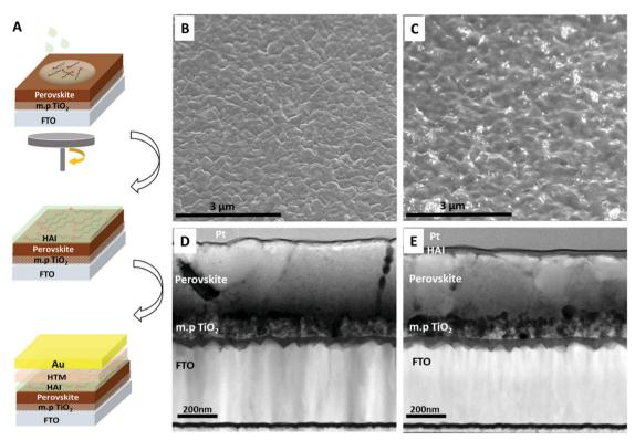
Fig. 1 (A) Schematic illustration of the HAI post deposition on top of crystallized 3D perovskite and the complete structure of the solar cell. Scanning electron microscopy (SEM) images of the perovskite surface (B) without HAI treatment and (C) after HAI treatment. Focused ion beam (FIB) cross section images of (D) the non-treated and (E) the HAI-treated samples. All samples are without hole-transporting material
