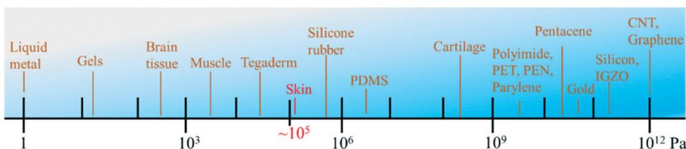
Fig. 2 Comparison of the elastic modulus values of electronic materials, polymers and biological materials.<sup>7</sup>
