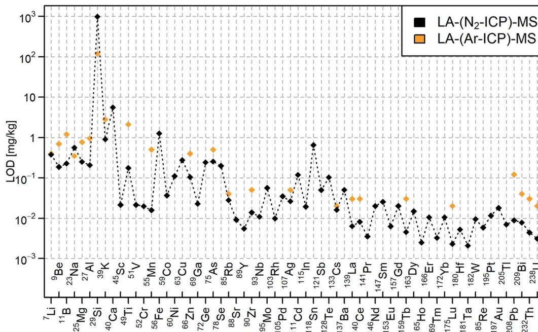
Fig. 4 LODs for NIST SRM 610 analyzed with LA- $(N_2$ -ICP)-MS (black) and LA-(Ar-ICP)-MS (orange) according to Günther *et al.*<sup>23</sup>
