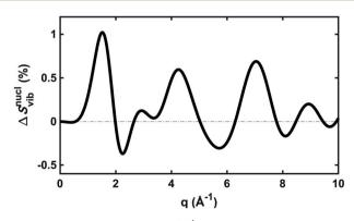
Fig. 4 The vibrational correction term,  $\Delta S_{\text{vib}}^{\text{nucl}}(q, \mathbf{R}')$ , for NMM in the 3s Rydberg state, assuming a vibrational temperature of 1000 K.
