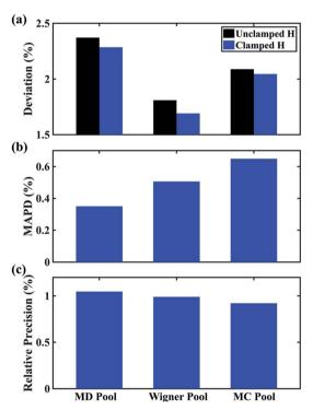
Fig. 6 Comparison of structure analysis results using three different structure pools. (a)  $\sum |\% \Delta S_{\text{exp}} - \% \Delta S_{\text{theory}}|$ The scattering pattern deviations calculated as and averaged
