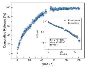
Fig. 4 MeJ release profile from nano-MeJ in aqueous solution containing 0.1% v/v of Tween-80. The dashed line represents the best fits of the experimental data to the first order equation:  $y(t) = a \times (1 - t)$  $e^{-kt}$ ), with the rate constant  $k = 0.05 h^{-1}$ . The inset shows the linearized experimental data (symbols) and the first order equation (line).
