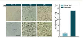
Fig. 6 (a) Optical micrographs of drops containing MeJ (top) and nano-MeJ (bottom) collected at different time intervals at 50 °C. Scale bar = 100  $\mu$ m. (b) Percentage of remaining MeJ (quantified by UV-vis spectroscopy) after 24 hours at 50 °C for both treatments.
