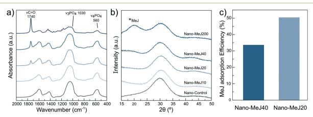
Fig. 1 (a) FTIR spectra and (b) XRD patterns of ACP nanoparticles (nano-Control) and nano-MeJ synthesized with increasing MeJ concentrations (nano-MeJ10, nano-MeJ20, nano-MeJ40 and nano-MeJ200). (c) MeJ adsorption efficiency for nano-MeJ40 and nano-MeJ20.
