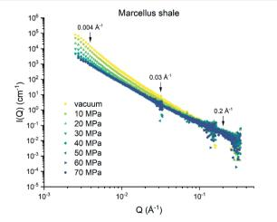
Fig. 1 Scattering intensity as a function of methane pressure for the Marcellus shale sample.
