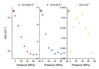
Fig. 2 Scattering intensity as a function of methane pressure at (a) Q of 0.004  $\text{Å}^{-1}$ , (b) Q of 0.03  $\text{Å}^{-1}$ , and (c) Q of 0.2  $\text{Å}^{-1}$  for the Marcellus shale sample.
