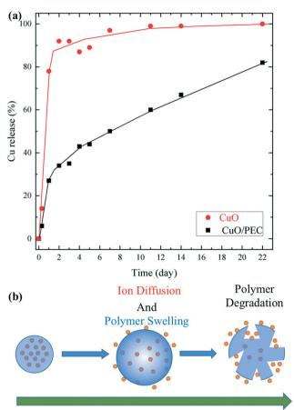
Fig. 6 (a) Cumulative percentage release of Cu versus time from CuO nanopowder and the CuO/PEC NPs, under a constant of pH = 5.5. (b) Schematic of the mechanism of Cu release from the CuO/PEC nanocomposite
