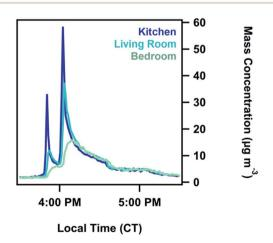
Fig. 3 Time series of a typical stir-fry cooking event, with data from the POPS in all three rooms monitored during the experiments. The left panel shows number concentration and the right panel shows mass concentration (using an assumed density of  $1.0 \text{ g cm}^{-3}$ ) over the course of the stir-fry.
