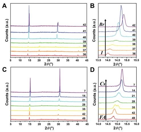
Fig. 4 XRD patterns of  $Cs_{1/6}FA_{5/6}Pb(Br_xI_{1-x})_3$  films as a function of the Br content (A and B) and  $Cs_yFA_{1-y}PbBr_3$  as a function of the Cs content (C and D). (B) and (D) are expanded views of the peaks at  $\sim 14-15^{\circ}$  in (A) and (B).
