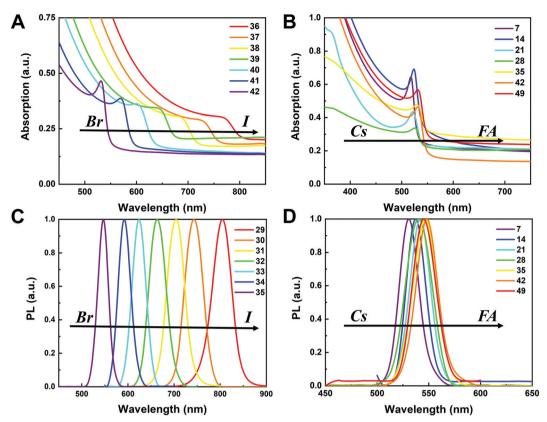
Fig. 8 Ultraviolet-visible absorbance spectra of  $Cs_{1/6}FA_{5/6}Pb(Br_{x}l_{1-x})_3$  (A) and  $Cs_{v}FA_{1-v}PbBr_3$  (B) films. Normalized photoluminescence spectra of  $Cs_{2/6}FA_{4/6}Pb(Br_xI_{1-x})_3$  (C) and  $Cs_vFA_{1-v}PbBr_3$  (D) films.
