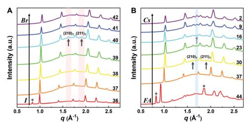
Fig. 5 Integrated circular average of 2D GIWAXS patterns for  $Cs_{1/6}FA_{5/6}Pb(Br_x|_{1-x})_3$  films as a function of the Br content (A) and  $Cs_yFA_{1-y}PbBr_{1/2}|_{5/2}$  as a function of the Cs content (B). δ-FAPbI<sub>3</sub> is marked by \*. The black arrows point to the characteristic peaks of the tetragonal phase and the grey arrow refers to the characteristic peaks of orthorhombic phase, i.e., (211)<sub>O</sub>, (121)<sub>O</sub>, (103)<sub>O</sub>.
