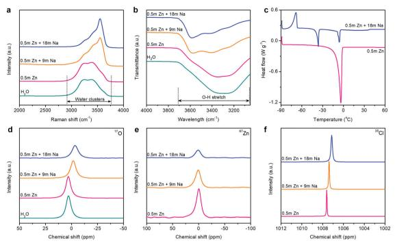
Fig. 2 Spectroscopic characterizations of the electrolytes. (a) Raman spectra, (b) FT-IR spectra, (c) DSC profiles, (d) <sup>17</sup>O (water) NMR spectra, (e) <sup>67</sup>Zn NMR spectra, and (f) 35Cl NMR spectra.
