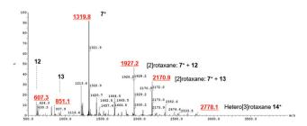
Fig. 7 ESI mass spectrum of crude reaction mixture showing formation of axle 7<sup>+</sup>, [2]rotaxane with macrocycle 12, [2]rotaxane with macrocycle 13 and hetero[3]rotaxane 14+.
