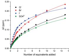
Fig. 3 Experimental titration data (points) and calculated 1:2 host: guest stoichiometric binding isotherms (lines) for the addition of anions as their TBA salts to XB rotaxane 11-PF<sub>6</sub> monitoring internal macrocycle proton β (CDCl<sub>3</sub>/CD<sub>3</sub>OD/D<sub>2</sub>O 45: 45: 10, 298 K, 500 MHz).
