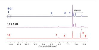
Fig. 6 Truncated <sup>1</sup>H NMR spectra (400 mHz, CDCl<sub>3</sub>, 298 K) of imidazolium-alkyne 5·Cl (top), an equimolar mixture of macrocycle **12** and 5·Cl (middle), and macrocycle **12** (bottom).
