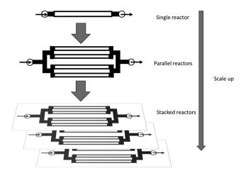
Scaling up and scaling out of µ-IMERs
