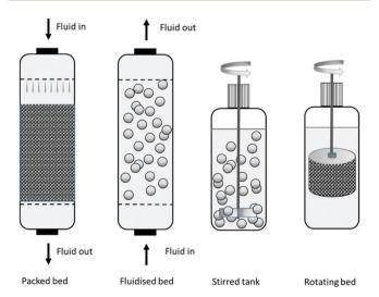
Fig. 8 Reactor design
