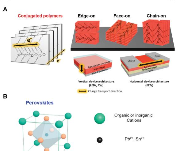
Fig. 2 Schematic illustration of solution-processable optoelectronic materials. (A) Structural representation of conjugated polymer (P3HT) with different molecular orientations (*i.e.*, edge-on, face-on and chain-on orientation) for different directions of charge transport and their corresponding optoelectronic applications. (B) Structural representation of perovskite, ABX<sub>3</sub> where A is methylammonium (MA), formamidinium (FA) or Cs, B is Pb or Sn, and X is Cl, Br or I.
