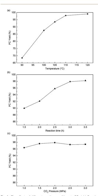
**Fig. 4** The effects of different reaction conditions to PC yield. Reaction conditions: PO (0.83 g, 14.3 mmol), HPIL-7 (180 mg, 1.5 mol%, based on the EA results), (a) 2 MPa CO $_2$ , 3 h. (b) 110 °C, 1.5 MPa (c) 110 °C, 3 h.
