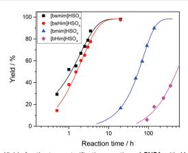
Fig. 5 Yields for the transesterification reaction of **PNPA** with MeOH at 25  $^{\circ}\text{C}$  measured from the UV-vis spectra at different reaction times for the four studied ILs. Lines are drawn for a better trend perception.
