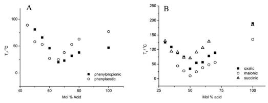
Fig. 4 Freezing points of five choline chloride-based DESs as a function of the composition. Reprinted with permission from ref. 22. Copyright (2004) American Chemical Society.
