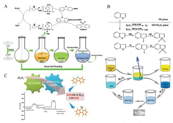
Fig. 9 The mechanism of extraction-oxidation desulfurization using DESs with H<sub>2</sub>O<sub>2</sub> as an oxidant. (A) L-Proline/p-TsOH DES system. Reprinted with permission from ref. 102. (B) ChCl/p-TsOH DES system. Reproduced from ref. 104 with permission from the Royal Society of Chemistry. (C) The reaction potential energy of the oxidation of glutaric acid with the assistance of acetamide. Reprinted with permission from ref. 39.
