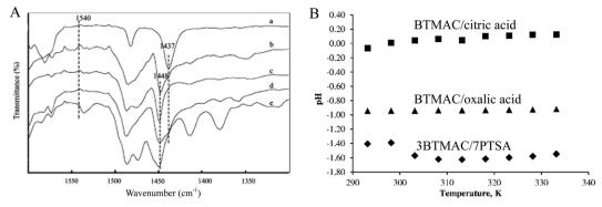
Fig. 7 (A) FT-IR spectra of (a) pure pyridine, (b) pyridine + choline chloride/ZnCl<sub>2</sub>, (c) pyridine + choline chloride/ZnCl<sub>2</sub>, (d) pyridine + choline chloride/ 3ZnCl<sub>2</sub> and (e) pyridine + benzyltrimethylammonium chloride/2ZnCl<sub>2</sub>. Reprinted with permission from ref. 60. (B) The dependence of pH on the temperature for three DESs. Reprinted with permission from ref. 62.
