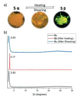
Fig. 7 (a) Photographs of the interconversion between polymorphs  $5\alpha$ and  $5\beta$  illuminated with a 365 nm lamp. (b) Thermal and subsequent mechanochromic polymorphic transformations followed by powder X-ray diffraction pattern changes.
