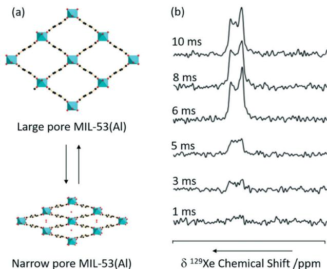
**Fig. 10** (a) 3D structure of MIL-53(Al) in exchange between the large and narrow pore form. (b)  $^1\text{H}$   $^{129}\text{Xe}$  CP spectra as a function of contact time under a MAS rate  $\nu_r = 8$  kHz at a temperature of 153 K and a pressure of 500 mbar. Reprinted (adapted) with permission from ref. 65. Copyright 2016 American Chemical Society.
