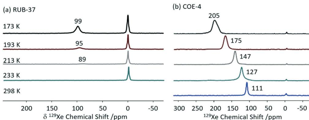
Fig. 8 Variable temperature hyperpolarised static  $^{129}\text{Xe}$  NMR spectra of (a) RUB-37 and (b) COE-4. Reprinted from ref. 63: structural investigation of interlayer-expanded zeolite by hyperpolarized  $^{129}\text{Xe}$  and  $^1\text{H}$  NMR spectroscopy, 109555, Copyright 2019, with permission from Elsevier.
