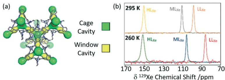
**Fig. 9** (a) Crystal structure of CC3 showing both cage cavities (yellow) and window cavities (green). (b)  $^{129}\text{Xe}$  NMR spectra of CC3 with varying xenon loadings (HL<sub>Xe</sub> – high loading, ML<sub>Xe</sub> – middle loading and LL<sub>Xe</sub> – low loadings) at 295 and 260 K. Reproduced from ref. 60 with permission from the PCCP Owner Societies.
