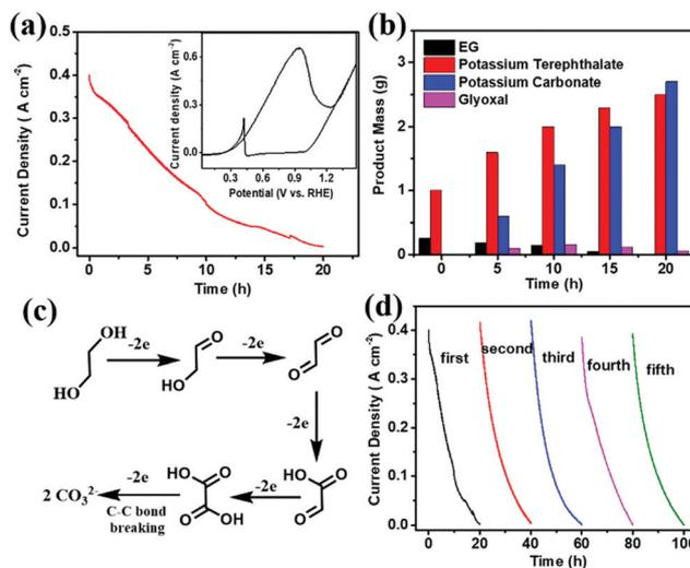
Fig. 3 (a) PET electro-reforming chronoamperometry curve on Pd/NF-10 at 0.7 V vs. RHE; inset: CV curve of the PET electroreforming substrate at a scan rate of  $10 \text{ mV s}^{-1}$ ; (b) product analysis of PET electroreforming on Pd/NF-10 at 0.7 V vs. RHE; (c) proposed reaction mechanism for EG oxidation on the Pd/NF-10 electrocatalyst; (d) stability test for PET electro-reforming on Pd/NF-10 at 0.7 V vs. RHE for 5 cycles.
