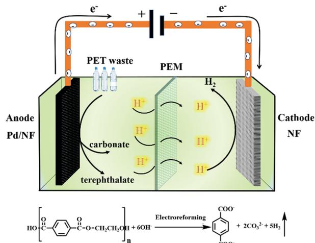
Scheme 1 Schematic illustration of the electroreforming of PET into high value-added chemicals and H<sub>2</sub> fuel.
