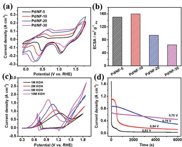
Fig. 2 (a) CV curves of Pd/NF in 1 M KOH solution at a scan rate of 10 mV s<sup>-1</sup>; (b) corresponding ECSA values of Pd/NF; (c) CV curves of Pd/NF-10 in alkaline EG solution (different concentrations of KOH + 1 M EG) at a scan rate of 10 mV s<sup>-1</sup>; (d) chronoamperometry curves of Pd/NF-10 in alkaline EG solution (10 M KOH + 1 M EG) under different potentials.
