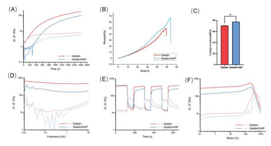
Fig. 2 Rheological properties of the gelatin and gelatin/HAP scaffolds. (A) The time sweeps. (B) Stress-strain curves. (C) Elastic modulus. (D) Frequency sweeps. (E) Shear thinning. (F) Strain sweeps of gelatin and gelatin/HAP hydrogel.
