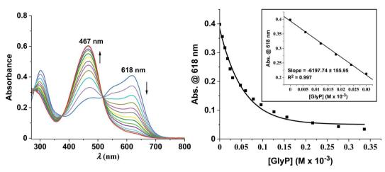
Fig. 5 Left: UV-vis spectra of titration of Zn<sup>II</sup>-zincon (30  $\mu$ M;  $\lambda_{max} = 618$  nm) with GlyP leading to metal-free zincon ( $\lambda_{max} = 467$  nm) at pH 7.20, [HEPES buffer] = 10 mM. Right: Corresponding calibration curve ([Zn<sup>II</sup>-zincon] = 30  $\mu$ M, [GlyP] = 0-30  $\mu$ M; LOD = 4.80  $\mu$ M (811  $\mu$ g L<sup>-1</sup>),  $R^2 = 0.997$ ).
