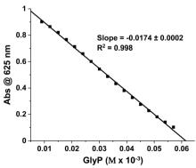
Fig. 6 Left: Changes of absorbance of Cu $_{\rm L}^{\rm U}$ -PV (30  $\mu$ M,  $\lambda_{\rm max}=625$  nm) in the presence of GlyP (0–60  $\mu$ M) at pH 6.50, [HEPES buffer] = 10 mM;  $\lambda_{\rm max}$  (PV) = 445 nm. Right: Calibration curve with an LOD of 2.50  $\mu$ M (422  $\mu$ g L $^{-1}$ ) ( $R^2=0.998$ ).
