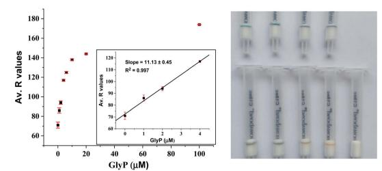
Fig. 8 Left: Averaged R values of calibration samples of immobilized Cu $_{-}^{\parallel}$ -PV (10 nmol; detection zone: blue) treated with different conc. of GlyP (2 mL; 0–100 μM; 0–200 nmol). Inset: Corresponding calibration curve: LOD\* = 2.66 μM (450 μg L $^{-1}$ ),  $R^2$  = 0.997. Right: A photograph of calibration samples (from top left to bottom right: 0–100 μM; bottom right: empty white cartridge).
