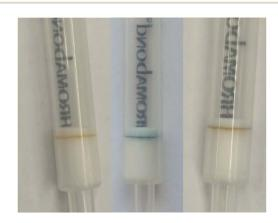
Fig. 7 Immobilizations of PV and  $Cu_{\perp}^{\parallel}$ -PV on the top of C18ec cartridges at pH 6.50 ([HEPES] = 10 mM). Left: PV (2 mL, 5  $\mu$ M; 10 nmol; dark yellow), middle:  $Cu_{\perp}^{\parallel}$ -PV (2 mL, 5  $\mu$ M; 10 nmol; detection zone: blue), right:  $Cu_{\perp}^{\parallel}$ -PV + GlyP (2 mL, 5  $\mu$ M, 10 nmol; detection zone: dark yellow).
