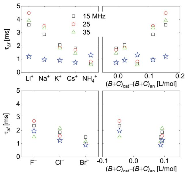
**Fig. 10** QCM response times,  $\tau_{\Delta f}$ , as determined from  $\Delta f(t)$  for the different ions. On the right-hand side, times are plotted versus  $\sum(B_i + C_i)/z_i$ . Stars ( $\star$ ) are RC-times as inferred from EIS. Fractional errors of the mean: cations : 2.4%; anions : 4.6%.
