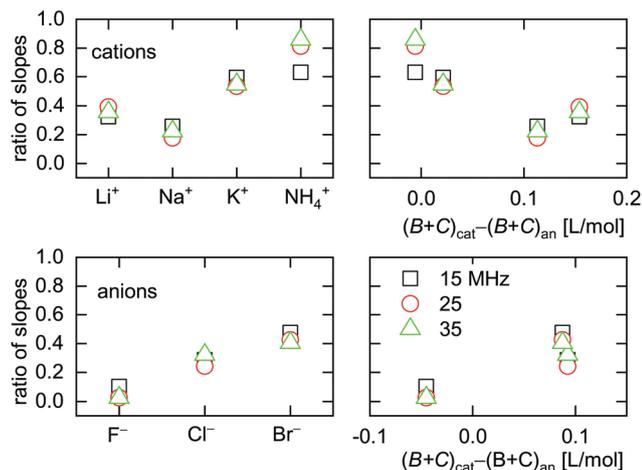
**Fig. 9** Ratio of slopes  $\langle A/\Delta E \rangle_{\Delta f} / (-\langle A/\Delta E \rangle_{\Delta f})$  as obtained from  $\Delta \Gamma$  and  $\Delta f$  (eqn (13)). Large ratios indicate a large elastic contribution.  $\text{Cs}^+$  was omitted from this graph because the sign of  $\langle A/\Delta E \rangle_{\Delta f}$  for  $\text{Cs}^+$  was opposite to the sign of  $\langle A/\Delta E \rangle_{\Delta f}$  for all other ions.
