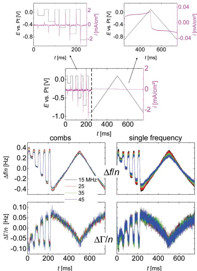
**Fig. 3** Typical raw data, consisting of a set of amplitude-variable square waves and two linear ramps. The sample was an aqueous  $\text{LiNO}_3$  electrolyte at a concentration of 20 mM.  $E$  vs. Pt is the electrode potential referenced to a platinum pseudo reference electrode.  $i$  in the top graphs is the current density.
