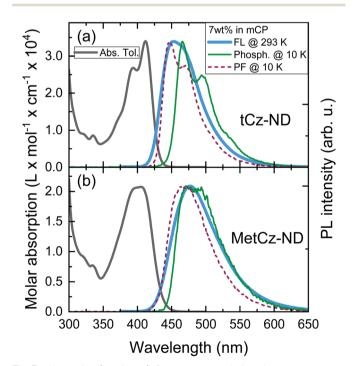
Fig. 3 Absorption (in toluene), fluorescence and phosphorescence spectra (in mCP, and an oxygen-free environment) of **tCz-ND** (a) and **MetCz-ND** (b) at room temperature and 10 K. Prompt FL spectra at 10 K are also shown.
