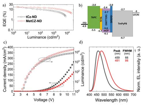
Fig. 5 Characteristics of vacuum-processed OLEDs based on the naphthyridine TADF emitters (7 wt% in mCP): (a) EQE vs. luminance, (b) energy level diagram, (c) current density and luminance vs. applied voltage, and (d) normalized electroluminescence spectra.
